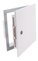
The dimension of the installation opening = the nominal dimension of the hatch Outside dimension of the lid = nominal dimension of the hatch +35 mm
