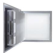
Sound insulation of PTL-dB hatches tested and classified Dn,e,w according to ISO 717-1:1996 PTL2020dB / 200\*200 -> 47 Dn,e,w[dB] PTL6060dB / 600\*600 -> 43 Dn,e,w[dB]
